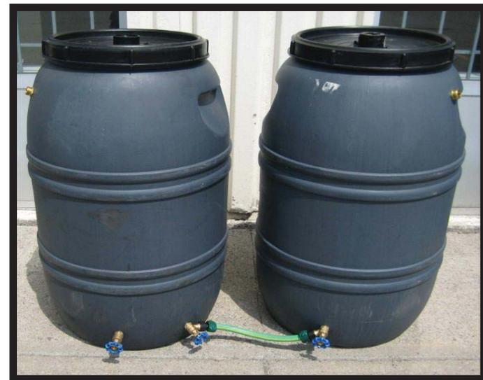
Barrels connected at the bottom
